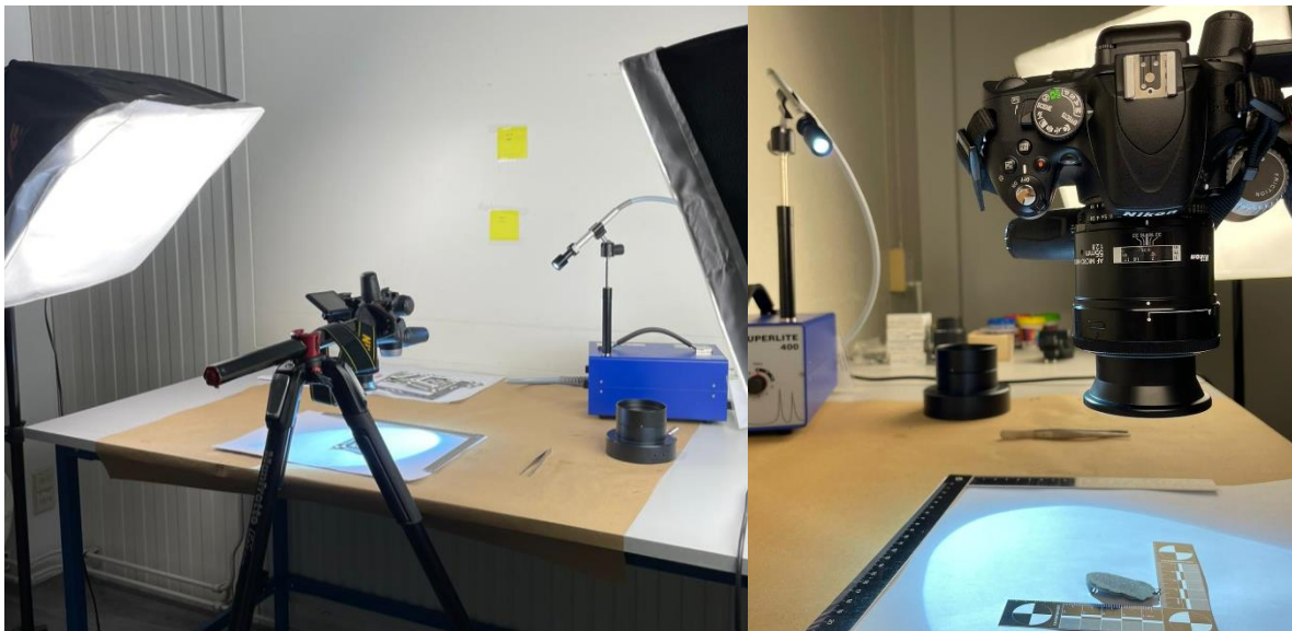
Figure 31 Photo set-up of the main research (left) general set-up with additional light sources (2x studio lamp, 1x lumiscene white light), captured with a Nikon D5100 with fixed settings and set-up (right) detailed image of the set-up with rulers and a white background.
