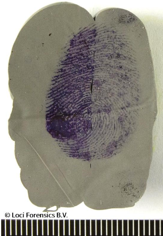
Figure 10 Forensic Sil winter version (left half-fingerprint) versus summer version (right half-fingerprint).
